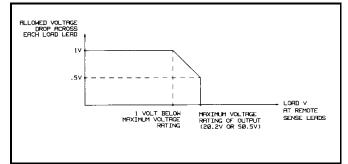
Figure 4-6. Allowable Load Lead Voltage Drop with Remote Sensing
